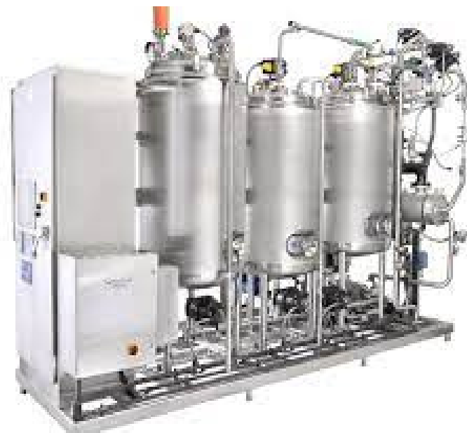
Automated CIP Skid for cleaning of mix vessel and connected accessories
