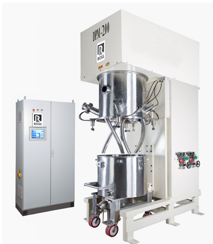
Double Planetary Mixer with High Viscosity Blades (US Patent No. 6,653,137)
